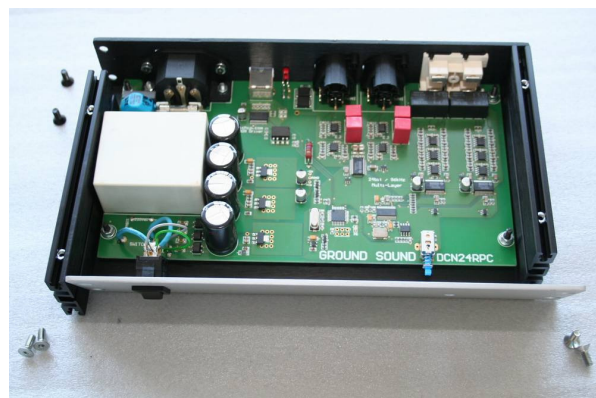
Glide Sides onto nuts on Bottom Plate Glide M3 Nuts into Sides – two in each Fix the Sides to Back Panel with M4x10mm black Mount Front Panel to sides with M4x10mm
