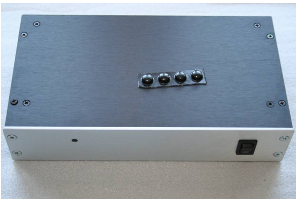
Flip over the chassis Tighten screws between sides and bottom plate
