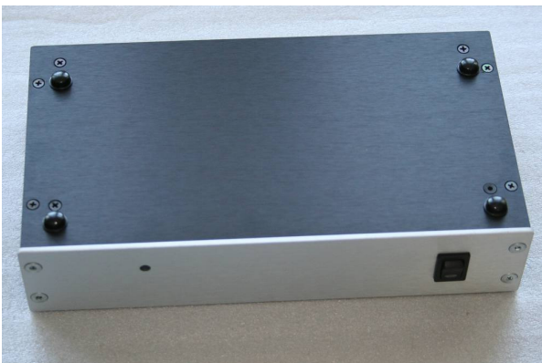
Mount Rubber feet Flip over again and tighten nuts on PCB
