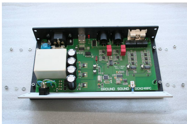
Mount PCB/BackPanel on Bottom Plate 3mm Washer / 3mm Spring Washer / M3 Nuts
