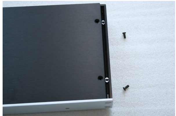
Align M3 nuts to holes in top plate Mount M3x8 screws
